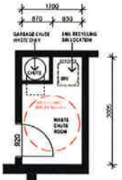
TYP WASTE CHUTE ROOM DETAIL SCALE 1:50
